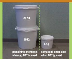
If you do not use these simple techniques to correctly empty the IBC, you may lose between 25 kg and 50 kg of remaining product in each IBC.
